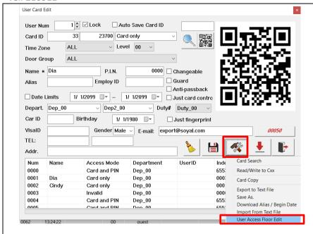
Step 1. After upgrading custom firmware for access controller, go to 701 Client 8. User Card Edit > Tool Box > User Access Floor Edit
