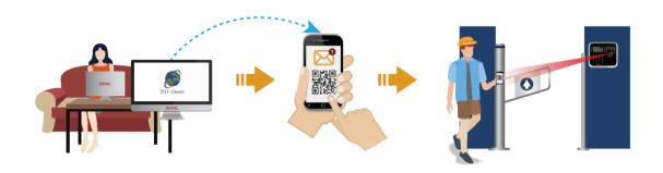
QRCODE access is easy to implement, access, and low in cost to create it, which is suitable for visitor management. 701 Client could convert card ID and generate it into QRCODE image and send the image to a designated e-mail. This could be use as limited time access identification to pass through a specific door groups, time and date limit (Eligible for Enterprise Series Controller). QRCODE will become invalid after expiration date and time.
