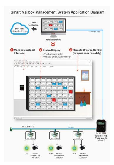
When letter or packages delivered to household's mailbox, the infrared I/O module installed in the mailbox detects the letter arrival and immediately sends signal to 701Client software installed at the management office through event log and at the same time if assigned personal email address is set could also send email notification to household. 701Client will also allow personnel to monitor which unit has letters or packages at one glance through Floor Plan feature.
